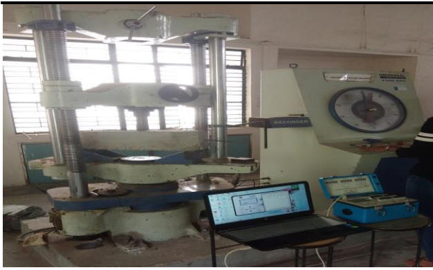
Figure no. 4.3- Experimental setup for calculation of strain and flexural strength.
