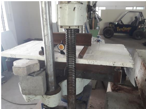
Fig.1 - Loading arrangement for flexural test.
