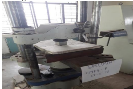
Fig.2 – Loading arrangement for punching shear test.
