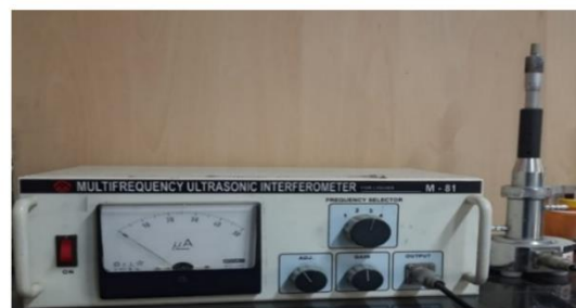
Figure 1: An ultrasonic Interferometer of 3 MHz frequency used for the purpose of irradiation.
