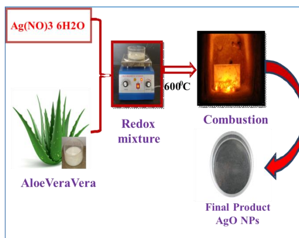
Fig 4.1. Schematic representation of the combustion synthesis of Silver Oxide nanoparticles
