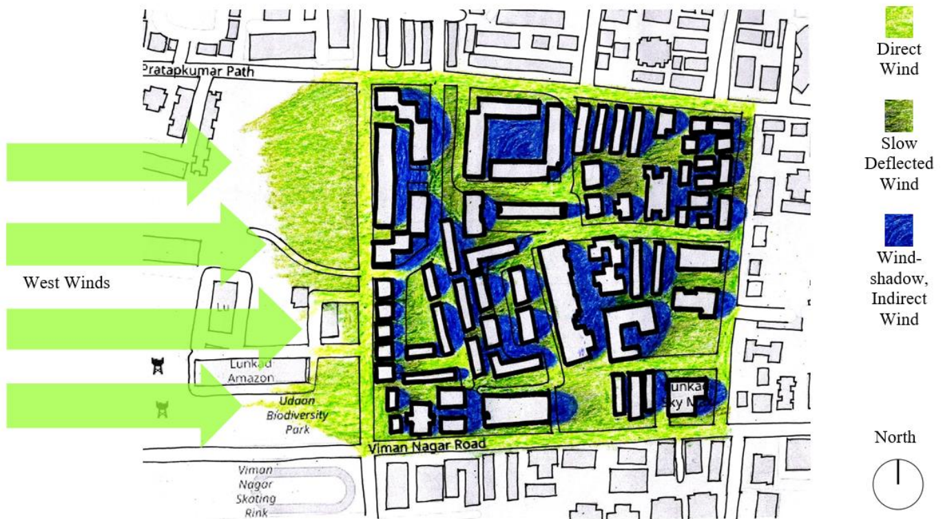
Fig.8: Wind and Wind shadow analysis of Vimannagar neighborhood, Pune using thumb rules, above 12m tree height (OpenStreetMap, 2021 for template map image)
