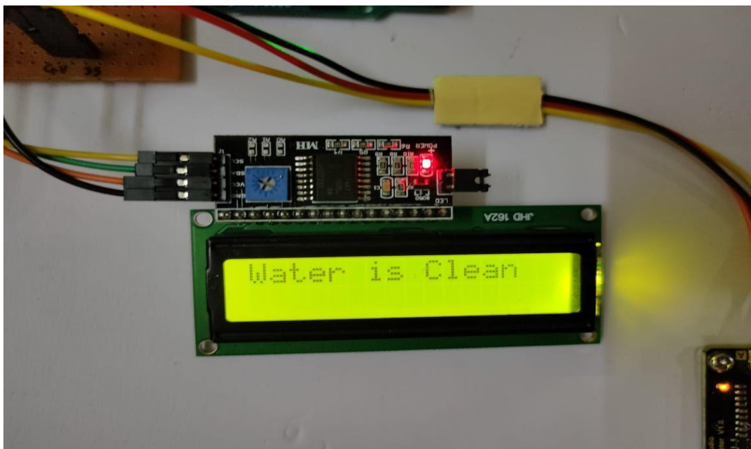
Fig. 11. Snapshot of LCD indicating purity of water
