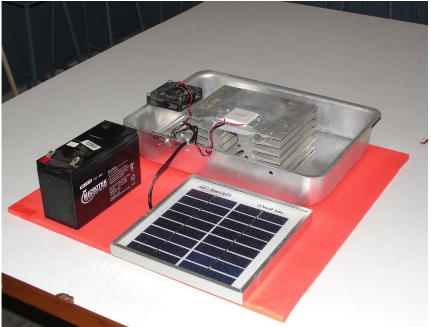
Figure 1.7: Final designed model of solar based thermoelectric refrigerator
