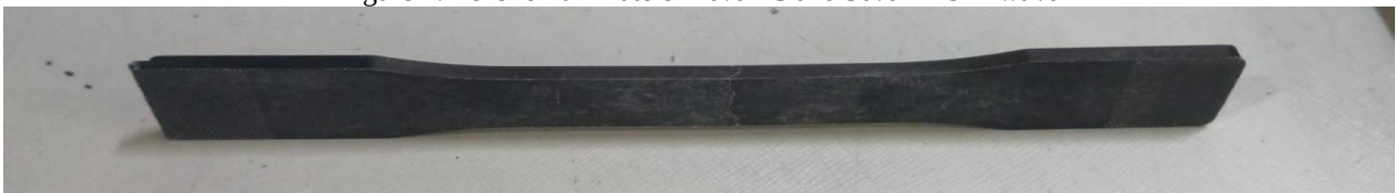
Figure 3: Tensile Laminate of 60% PC and 40% ABS in wt %
