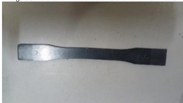
Figure 4: Tensile Laminate plain PC without blends
