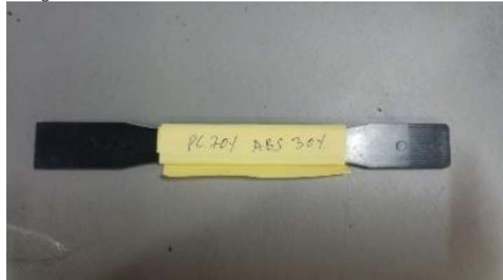
Figure 2: Tensile Laminate of 70% PC and 30% ABS in wt %
