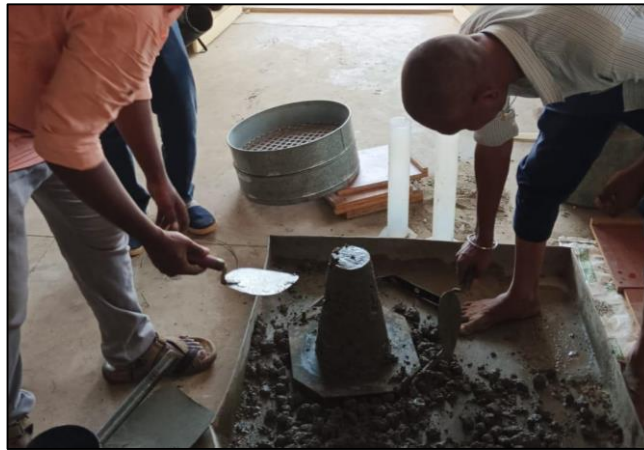
Figure 5.1: Slump test of Concrete
