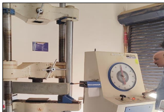
Figure 5.4: Flexural strength test
