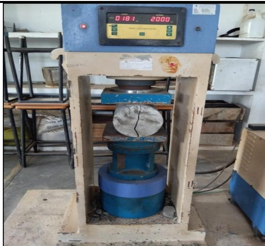
Figure 5.3: Tensile strength test
