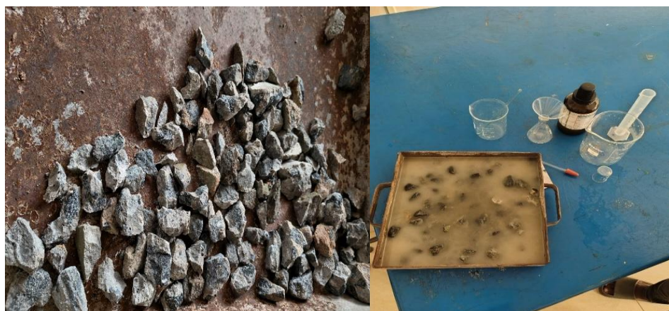
Figure 4.1: Recycled Aggregate (Demolished Concrete) and treating with HCL solution
