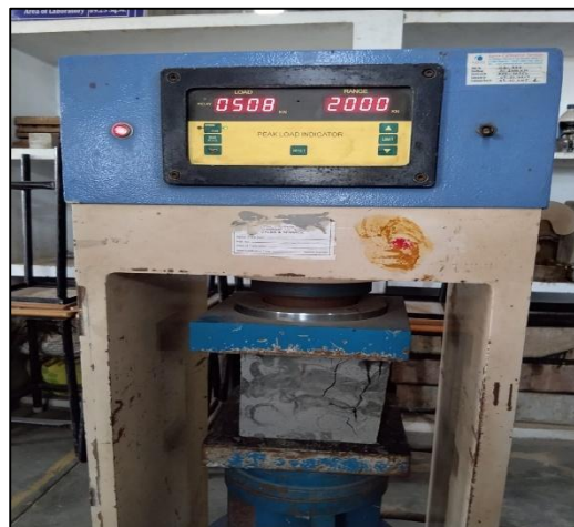
Figure 5.2: Compressive strength test
