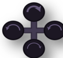
Fig 1: A quad rotor applying equal thrust in all the four rotors to lift in air or to maintain an altitude.
