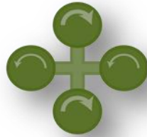
Fig 3: A quad rotor applying more thrust to one rotor and less thrust to its diametrically opposite rotor for adjusting its pitch.
