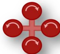
Fig 1: A quad rotor applying equal thrust in all the four rotors to lift in air or to maintain an altitude.
