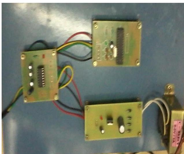
Figure.3 Photograph of wireless receiver module
