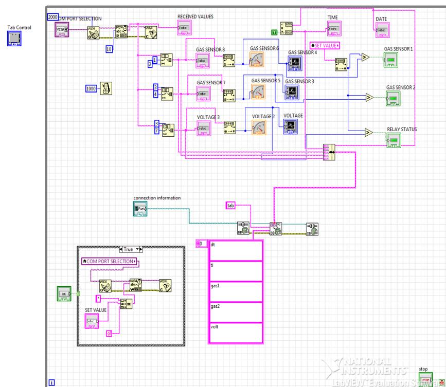
Figure.5 Block diagram of gas monitoring and control unit in LabVIEW
