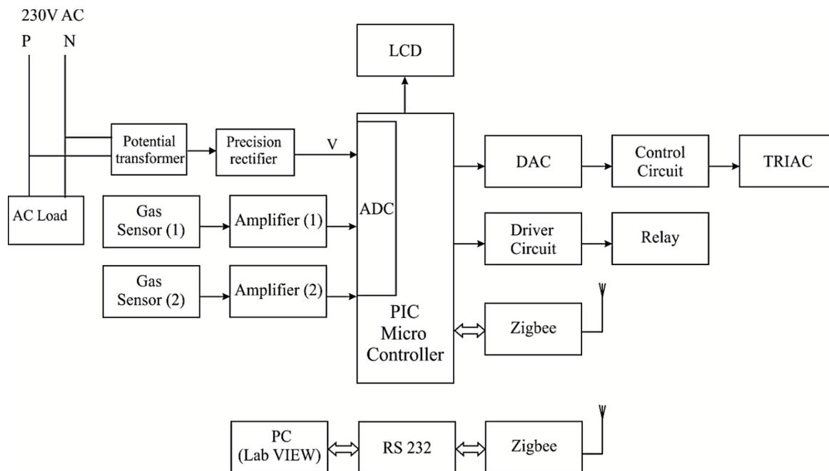
Figure.1 Block diagram of monitoring and controlling unit
