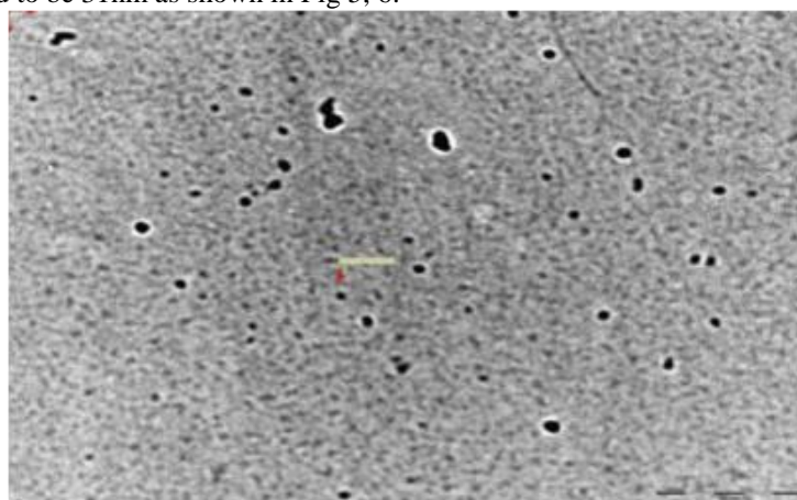
Fig 5: TEM micrographs of Silver nanoparticles synthesized using Curcuma amada
