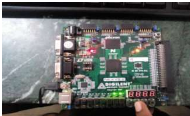
Figure 7. FPGA implementation of ALU operating in subtraction operation
