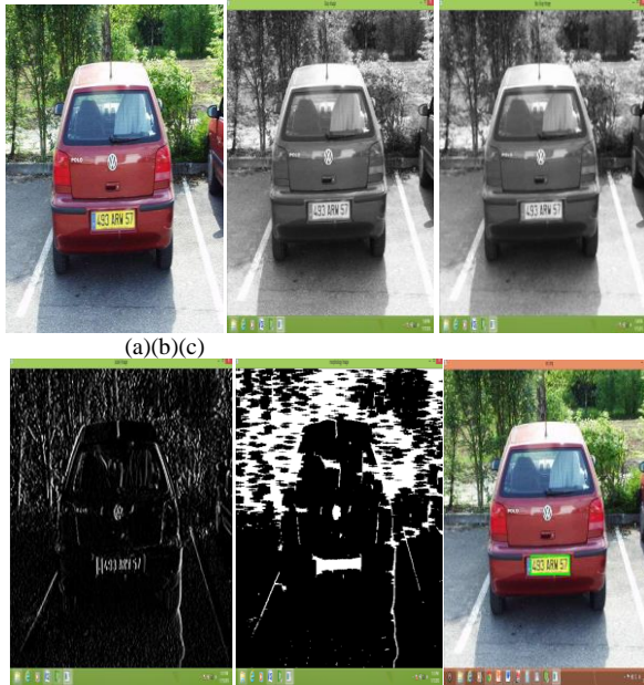
(d)(e) (f) Figure 3a) InputImage 1, b) Gray Scale Image, c) Median filtered Image d) Edge Detected Image,e) After applying Morphological operations,f) Plate Detection.
