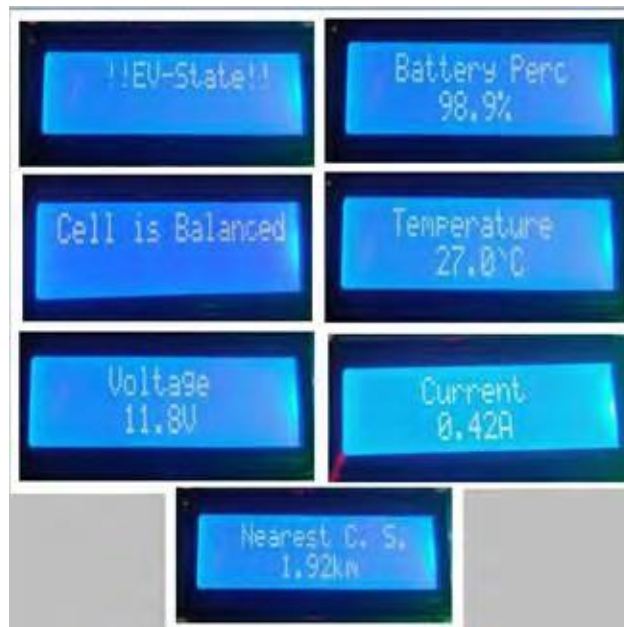
Fig.8. Data of battery charge, voltage, current temperature in LCD Display
