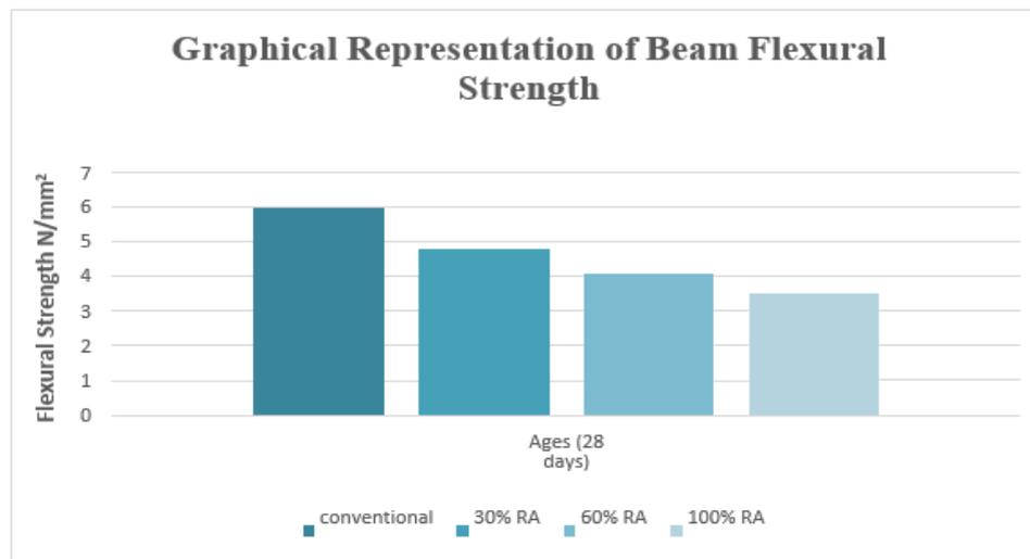
Figure 3: Flexural strength of concrete
