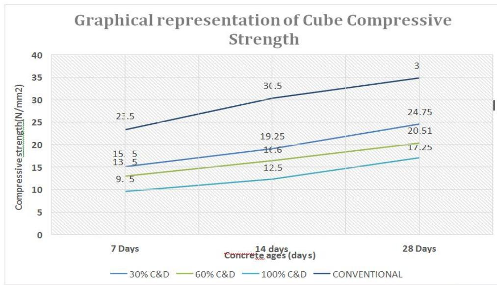
Figure 2: Compressive strength of concrete
