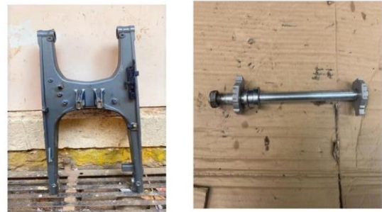
Fig. 7. Fabricated steel swing arm (left) and rear axle rod assembly (right).
