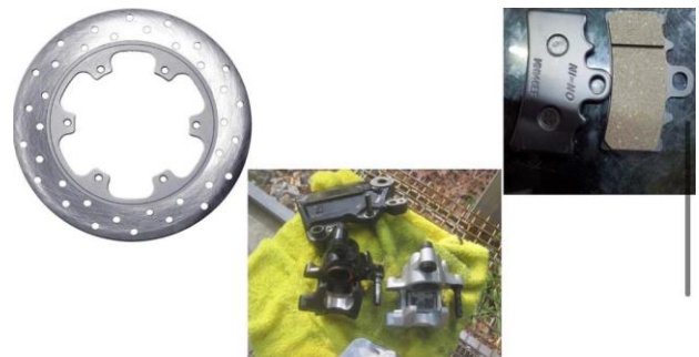
Fig. 8. Disc brake plate, brake pads, and hydraulic caliper assembly.
