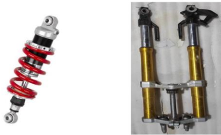
Fig. 4. Rear mono-shock absorber (left) and front telescopic fork assembly (right).
