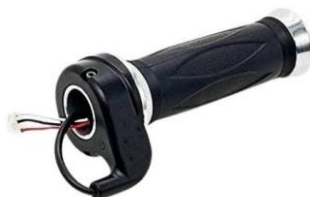
Fig. 11. Hall-effect twist throttle mounted on the handlebar.
