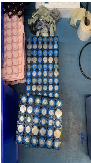
Fig. 9. NMC cylindrical cells arranged in the 20S 6P battery pack configuration.
