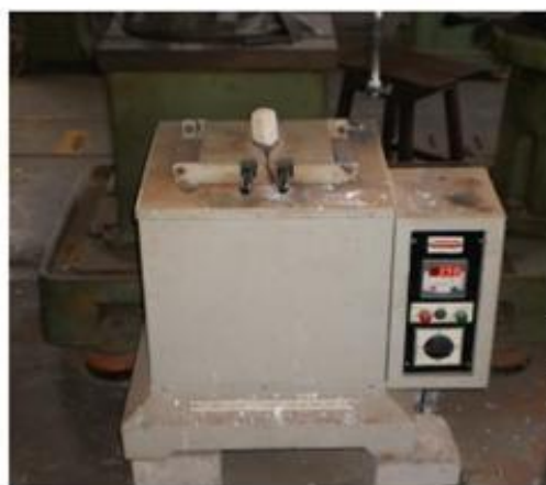
Figure 5: Muffle furnace and Preparation of samples
