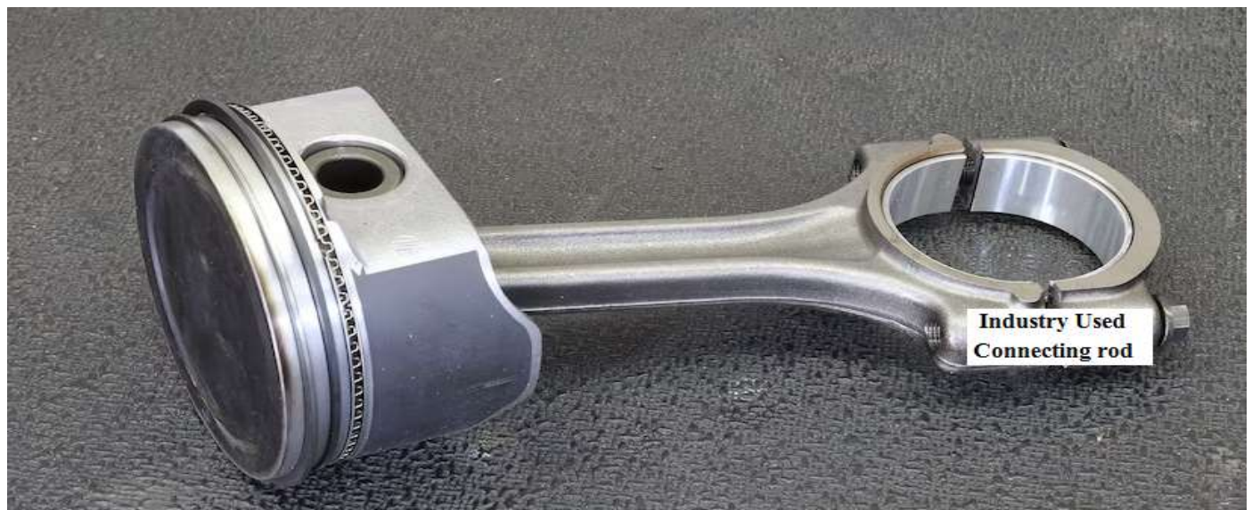
Fig. Industry Used Connecting Rod Made up of Steel
