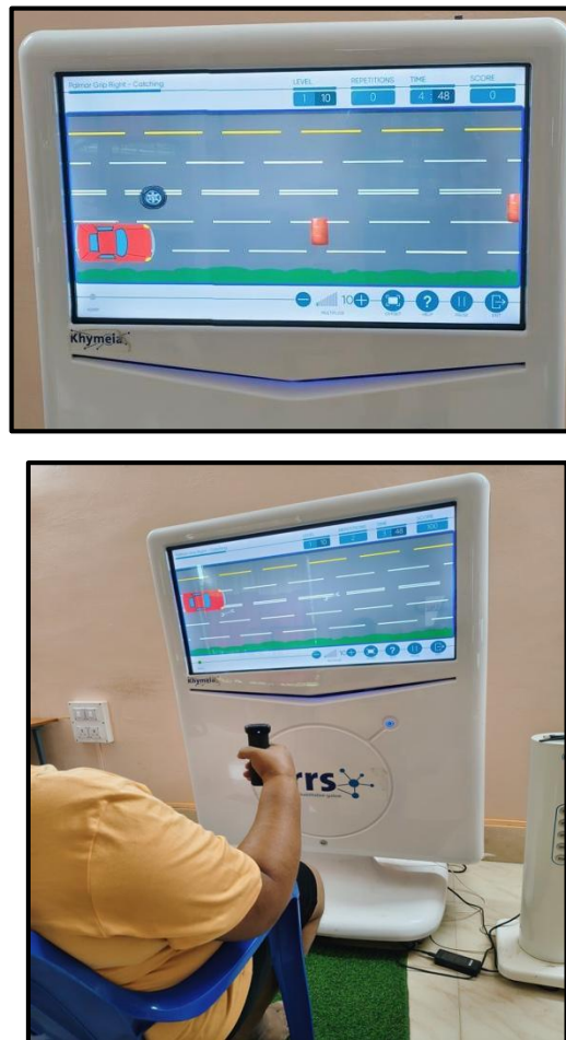
Fig. 8- Patient squeezes the K-force Grip sensor to control the car and collect the items.
