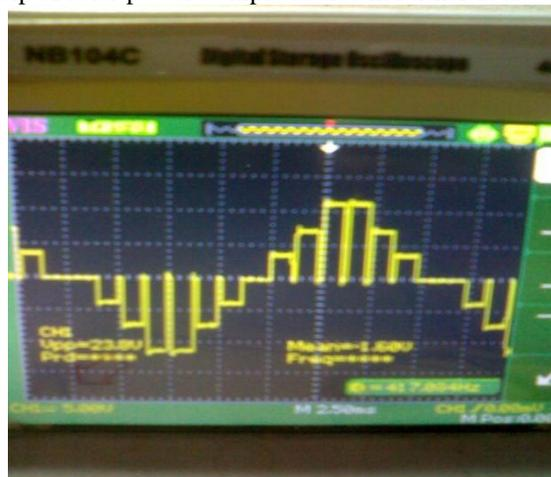
Fig 7:- experimental generated 5-level wave form of PWM inverter
