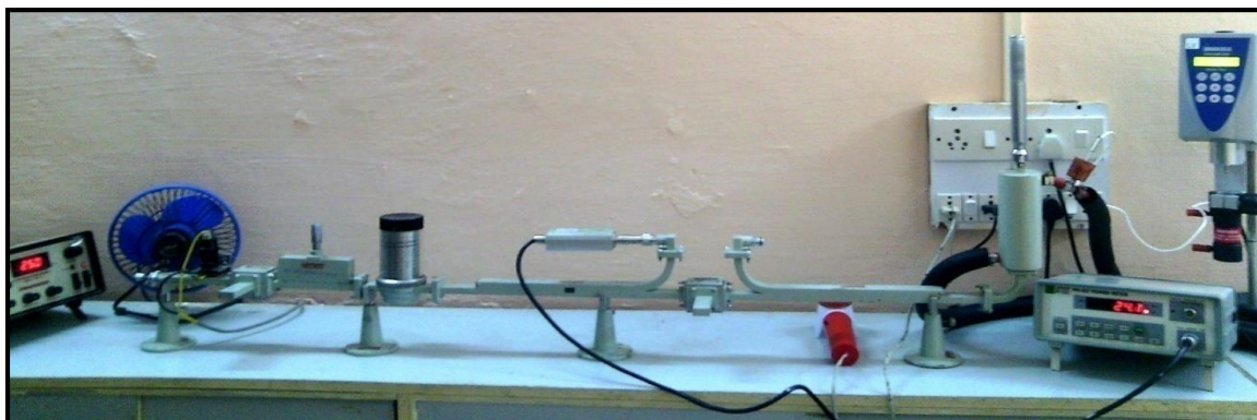
Figure 1. The experimental setup of microwave X-band bench for the measurement of \epsilon' and \epsilon''
