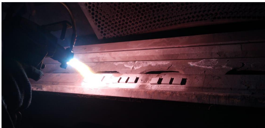
Fig. 4: Plasma spray coating event
