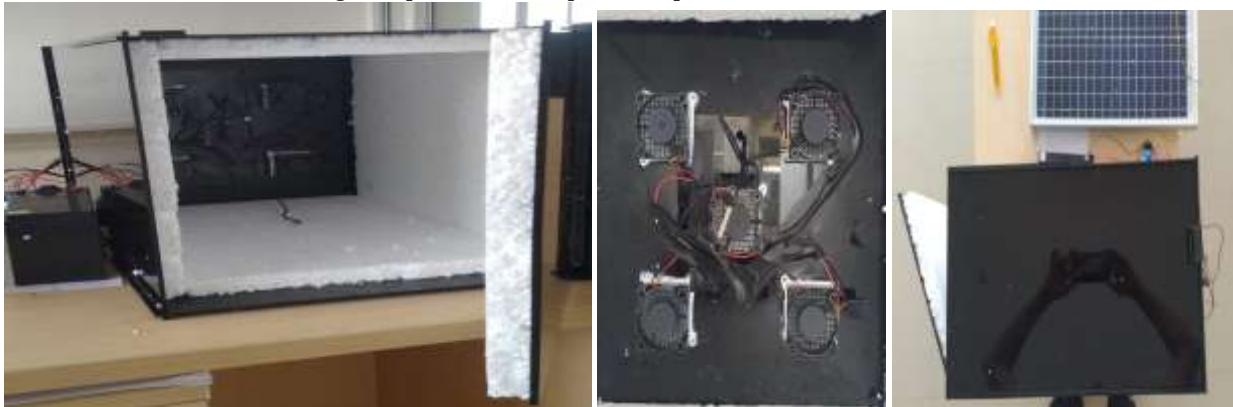
Fig 6: experimental setup of solar powered air conditioner
