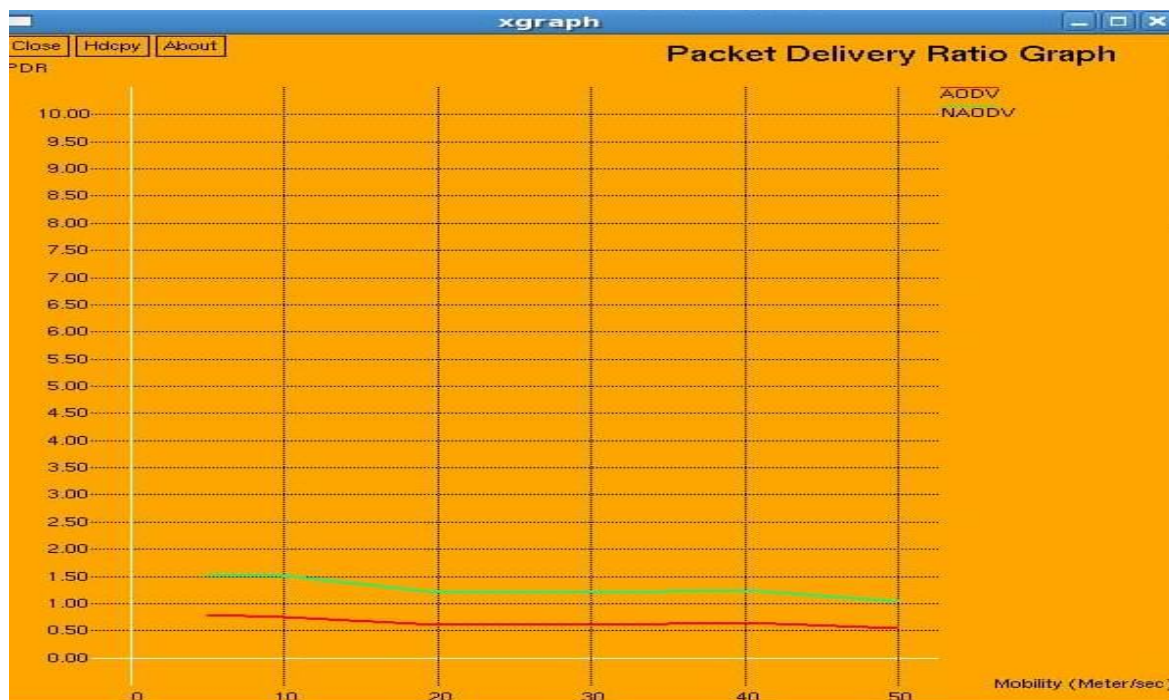
Fig 2: Energy Efficient AODV(marked as NAODV)V/S AODV Packet Delivery Ratio analysis at node 25
