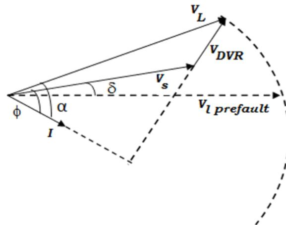
Fig: Vector diagram of phase advance compensation
