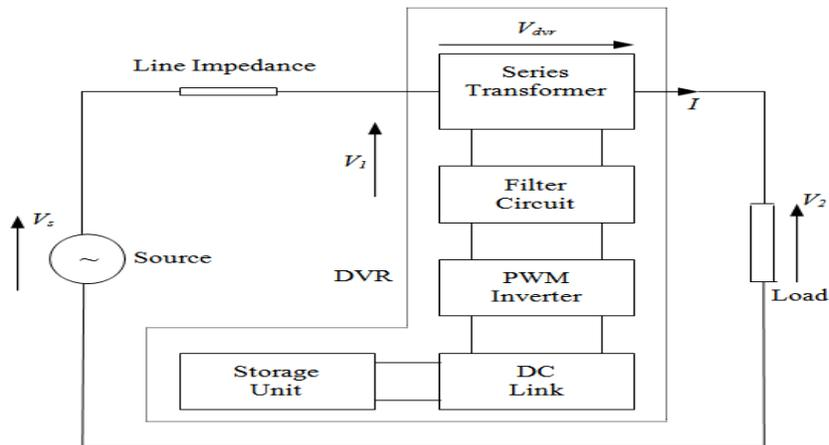
Fig2: Schematic diagram of Dynamic Voltage Restorer
