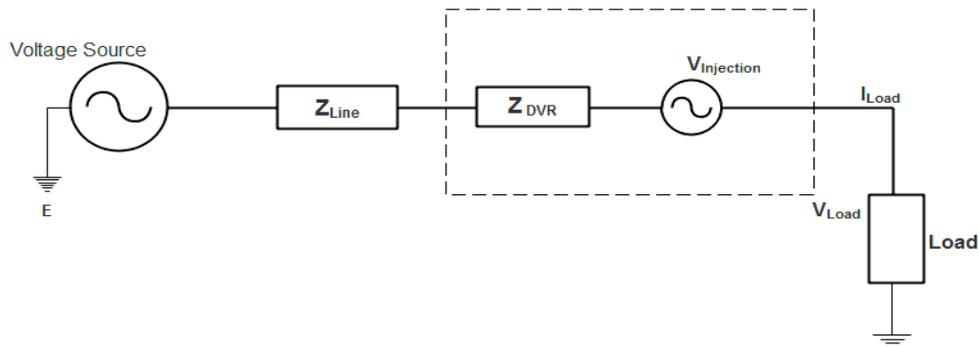
Fig1: Equivalent diagram of DVR
