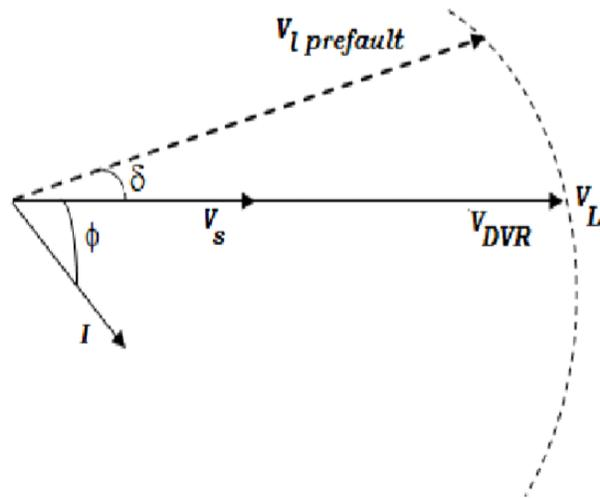
Fig: Vector diagram of in-phase compensation
