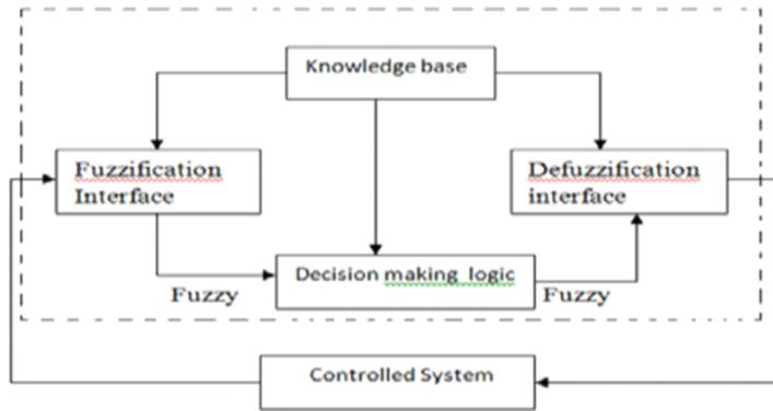
Fig: Basic structure of Fuzzy Logic Controller
