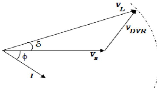
Fig: Vector diagram of pre-sag compensation
