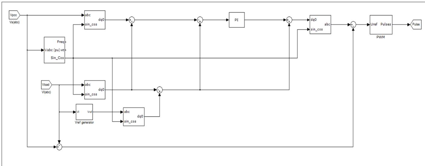
Fig: PI Controller for DVR
