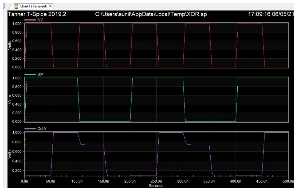
Figure3b.Simulation of GDI XOR gate
