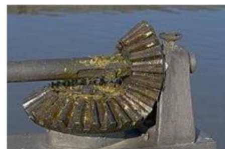
Fig 1.7 Bevel gear operating a lock gate
