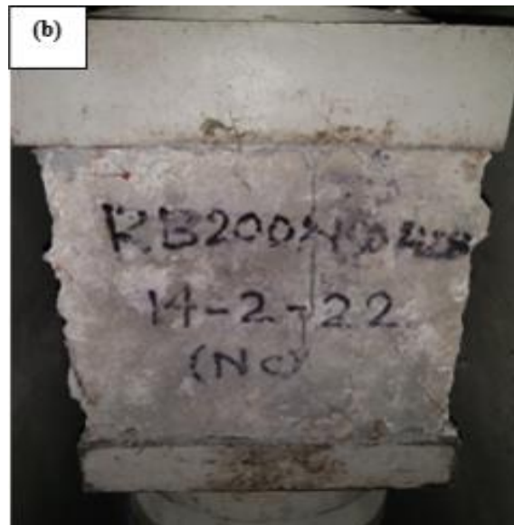
Figure 3 compressive strength test- (a) specimen heated in furnace, and (b) specimen under compression test
