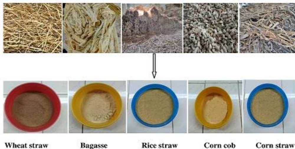
Fig. 1 Preparation of biomass sample from agricultural waste
