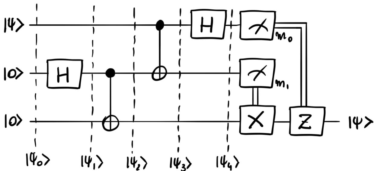
This is the quantum circuit for a quantum teleportation protocol where  $|\Psi_0\rangle$ ,  $|\Psi_1\rangle$ ,  $|\Psi_2\rangle$ , etc are the quantum state of the 3-qubit system at that point in time. Let the arbitrary qubit  $|\Psi\rangle = a|0\rangle + b|1\rangle$
