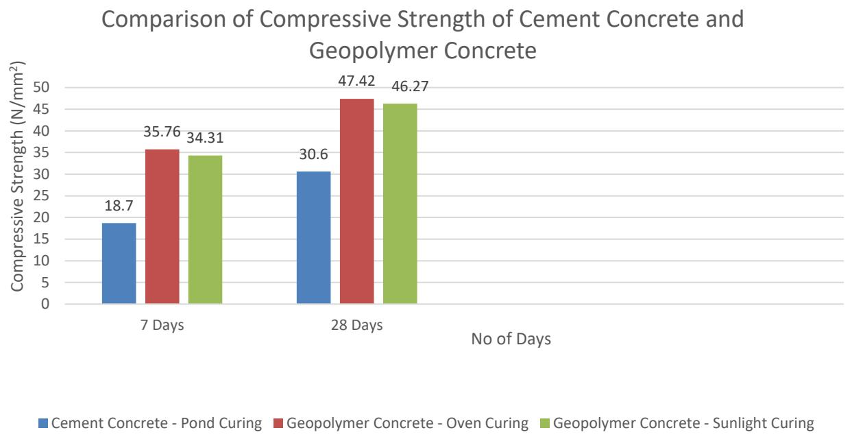
The compressive strength results for different curing methods are as follows:
