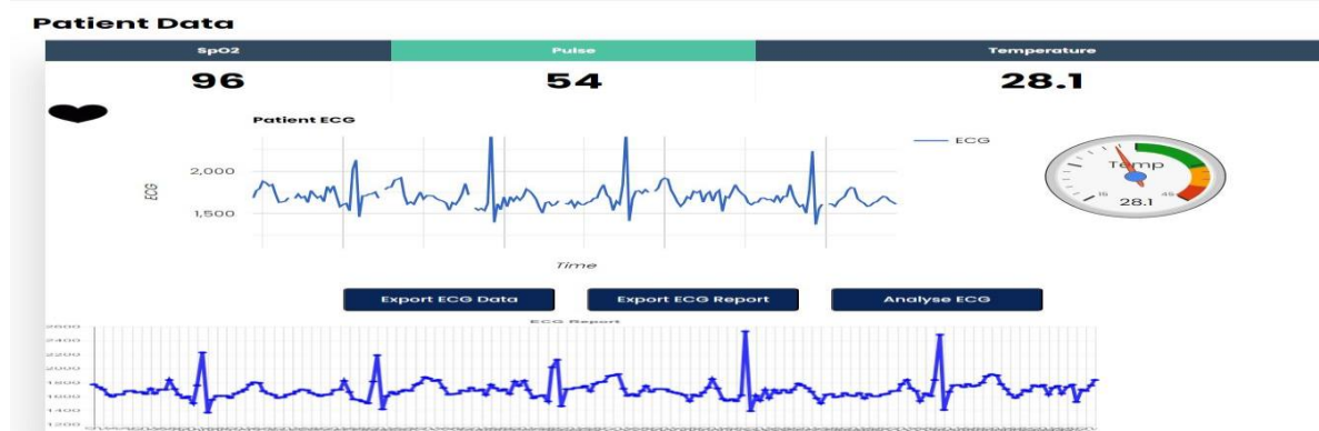
Fig. 10: Cloud-based web interface for real-time health tracking - Live patient health data such as body temperature, SpO2, heart rate and ECG can be viewed, tracked and analysed
